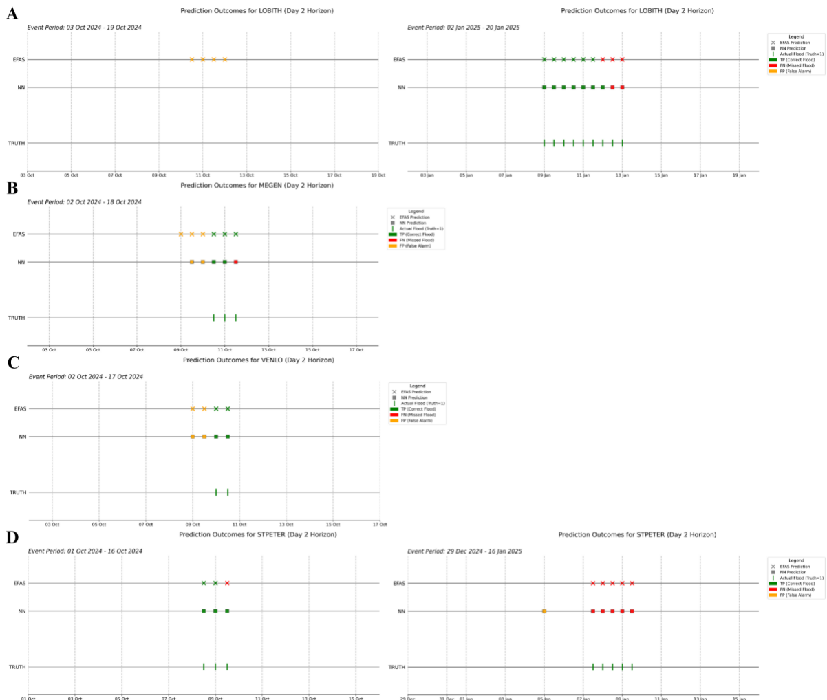
Figure F1. Temporal comparison of flood prediction outcomes at day 2 forecast horizon across four river gauging stations. The timelines show the performance of the operational EFAS system (top row crosses) and the ML model (middle row squares) against the observed Ground Truth (bottom row vertical markers). Panels display selected high flow period for Lobith (A), Megen (B), Venlo (C), St. Peter (D). Colour indicates classification performance, with green being TP, oranges being FP and red FN.
