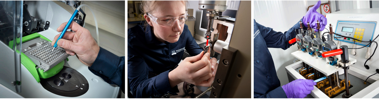
Figure 9: pictures of different thermal analytical techniques. From left to right: DSC, DMTA and HDT.
